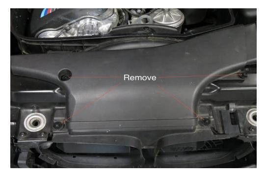
**Step 2-** Remove Secondary air dam elbow which connects to factory air box by taking each side of the elbow and pulling up.
