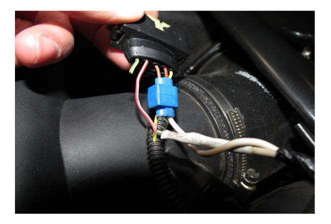
(Note- Here we soldered and heat shrink wrapped pin 1 wire to air intake temp harness wire. Feel free to do the same if you are confident with soldering.)
