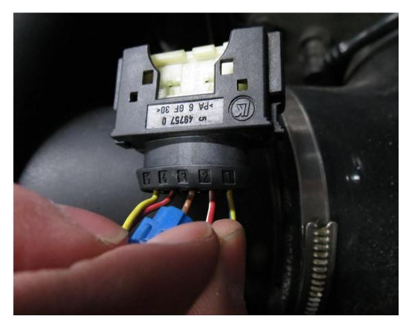
**Step 6:** Cut pin 1 wire, use provided butt connector to connect pin 1 wire to one of the two wires from air intake temp harness. (Note- The wire color on the Air Intake Temperature harness isn't important either of the two wires can be connected.) Once completed, use the vampire connector to piggyback the remaining air intake temp harness wire to pin 3.
