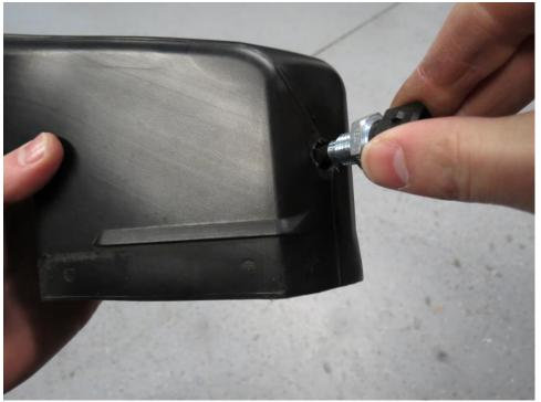
Once sensor is installed, install locking nut on the inside of air dam elbow using an open end and pliers or vise grips.
