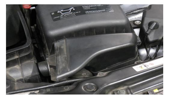
**Step 3-** Using a drill and 29/64 inch drill bit, drill a hole in the center of the right side of the plastic air dam elbow. (*Note- Make sure to remove all plastic shavings before moving on to the next step.*)
