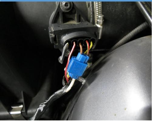
**Step 8**- Reinstall the secondary air dam elbow with the *TTFS* AIT sensor installed. Connect the TTFS AIT connector to sensor, reinstall intake air dam and 4 push pin clips.
